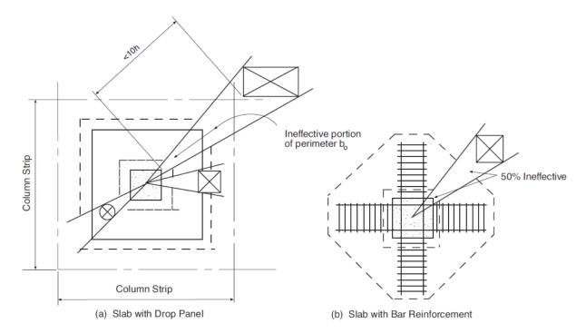
Figure 3 - Effect of Openings on Slabs Shear Strength (PCA Notes on ACI 318-11)
