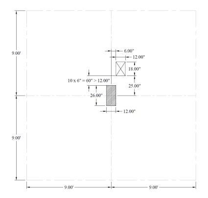
Figure 2 - Floor Opening Dimensions and Location
