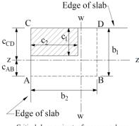
Critical shear perimeter for corner column
