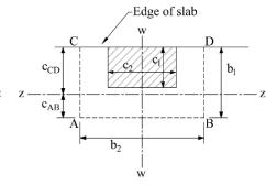
Critical shear perimeter for interior column
