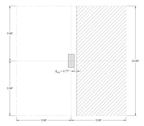
Figure 5 - Critical Section for One-Way Shear (Slab without Opening)
