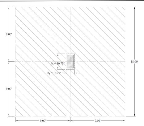
Figure 8 – Critical Section for Two-Way Punching Shear (Slab without Opening)
