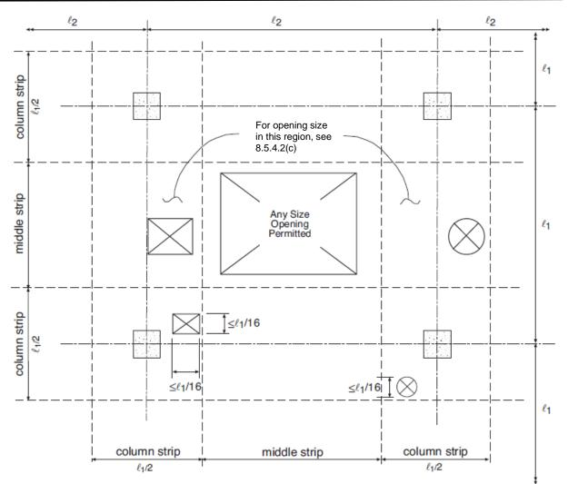
Figure 10 – Permitted Openings in Slab Systems without Beams for  $l_2 > l_1$  (PCA Notes on ACI 318-11)
